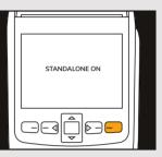
Press **ON** to put the card machine into standalone mode. The card machine will display 'STANDALONE ON'.
